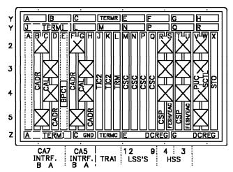
3. Remove the dummy cards or bypass card from identified adapter card(s) position and install the CSC card.
